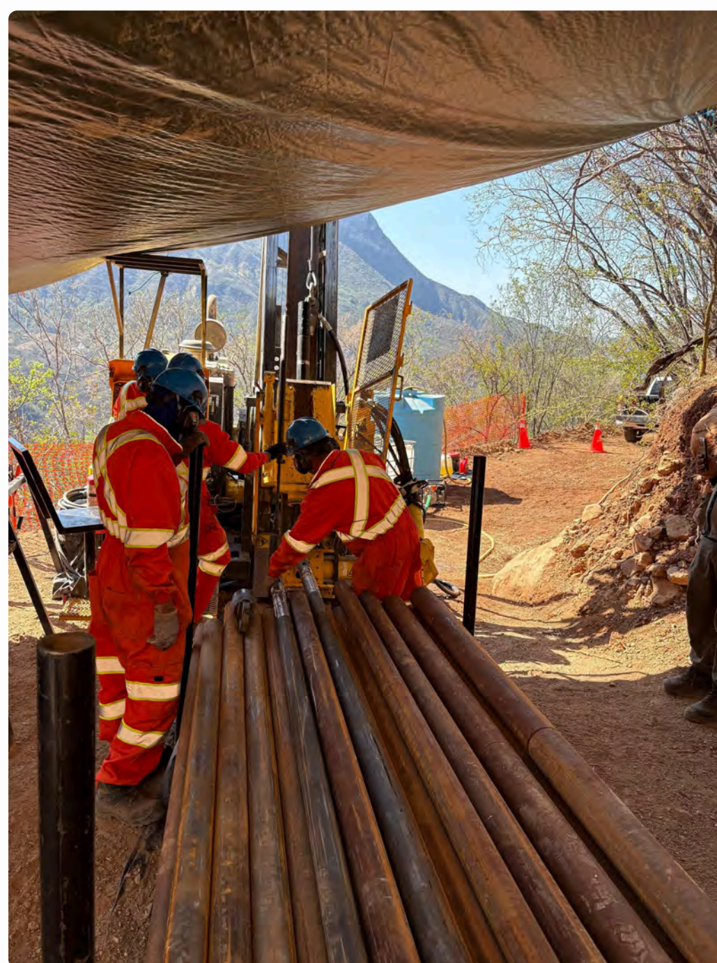
Drill crew operating the diamond drill rig at the Santo Tomás South Zone
