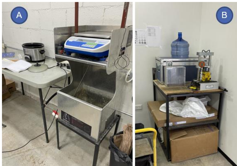
Figure 11-3: A: Specific Gravity Displacement Weight Equipment and Paraffin Wax Pot; B: UCS Point Load Tester
