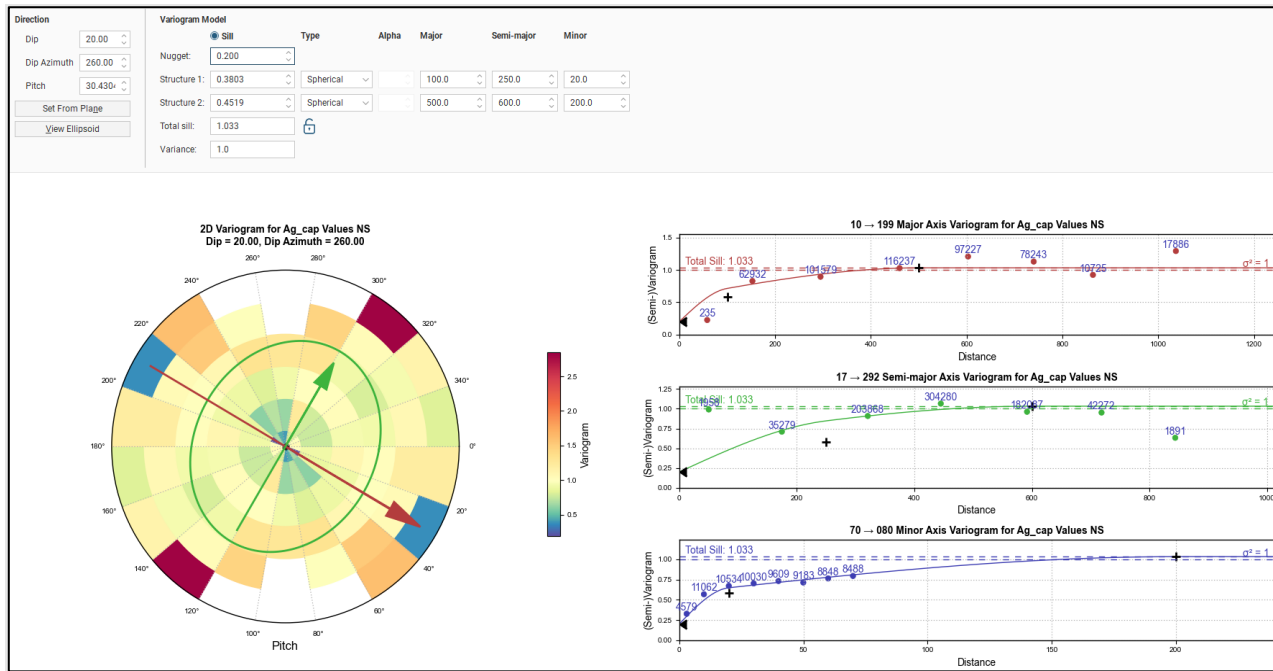
Figure 14-24: Normal Score Transformed Modelled Semi-Variogram for Ag in South Zone
