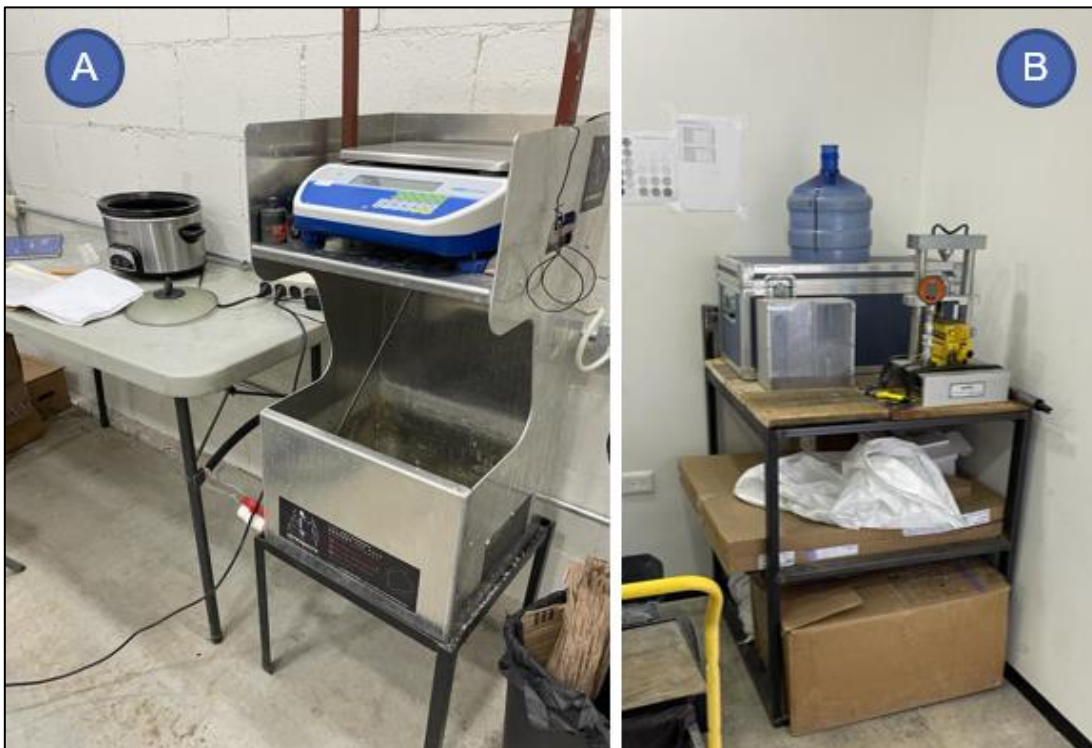
Figure 11-3: A: Specific Gravity Displacement Weight Equipment and Paraffin Wax Pot; B: UCS Point Load Tester
